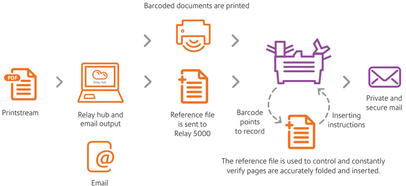
The reference file is used to control and constantly verify pages are accurately folded and inserted.
